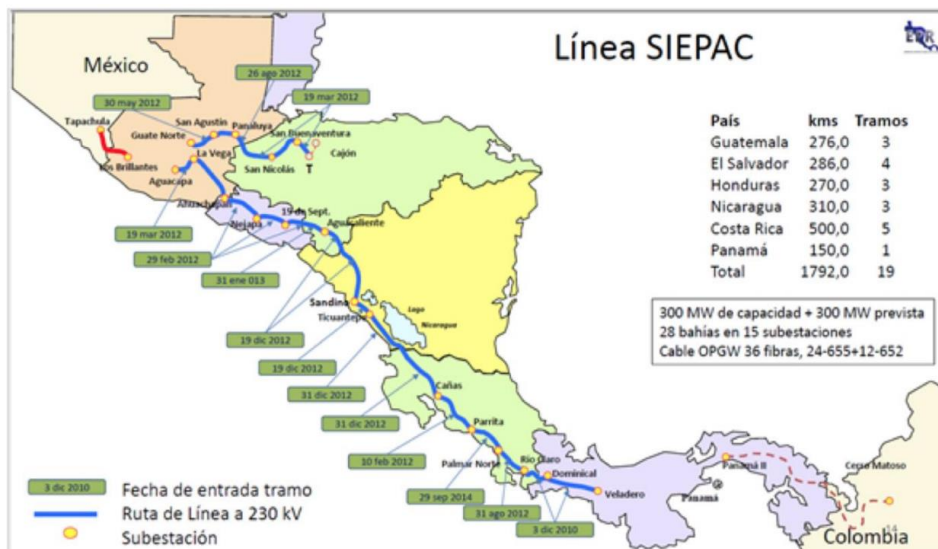
Figure 1. SIEPAC transmission line.
