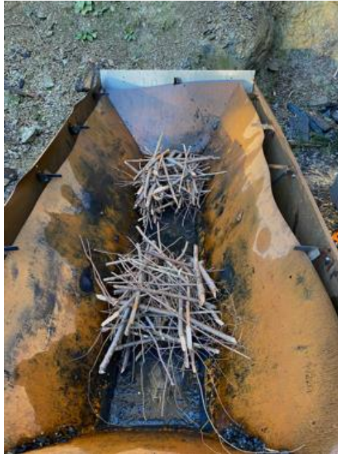
Figure 8. kindling material placed in the kiln.
