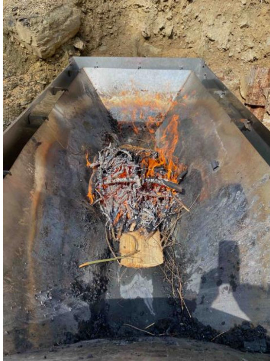
Figure 9. Kindling ready to be spread out and fresh feedstock added on top. In this case, the kiln was still quite wet at its base from a previous operation and the kindling was set up on top of a piece of wood, but this is not generally necessary.
