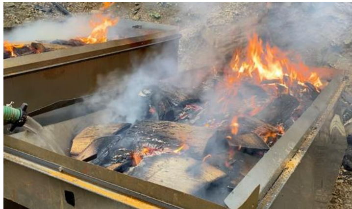
Figure 16. Pouring in quench water (gravity fed).
