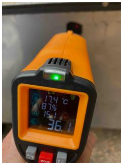
Figure 14. Despite the very high temperatures within the kiln, the shield walls should remain much cooler and safe to touch. In this case 36.1 °C was recorded. This is due to the strong upward flow of air between the kiln and shield walls. A matt black patch has been painted on the wall where the measurement is being made, to improve the accuracy of the IR temperature reading, relative to the reflective metal shield itself.
